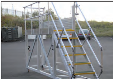
Flask inspection platform
